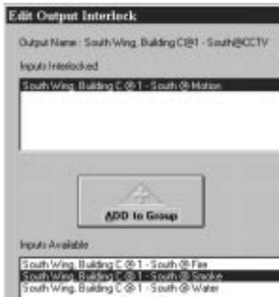
Figure 12. Interlocking Output Points to Input Points
